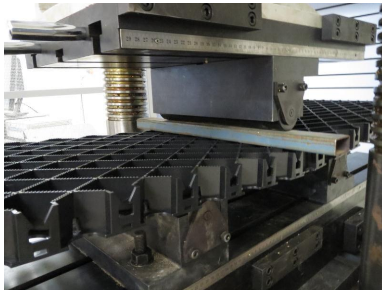
Figure 2. Flexural test at joints
