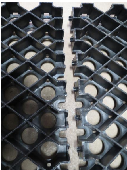
Figure 11. Failure of the joints
