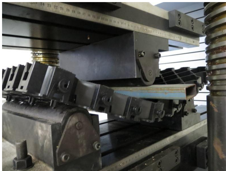
Figure 6. Deflection of the grid
