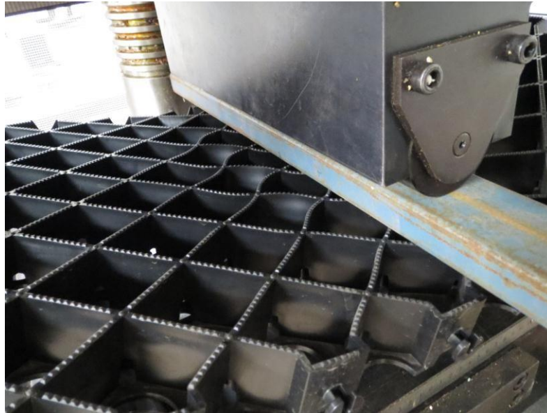
Figure 5. Deformation of the grid in compression
