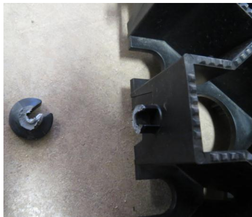
Figure 11. Failure of the joints
